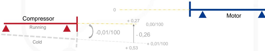
Vertical movement, Cold to Running (Off-line to Running condition, OL2R)
