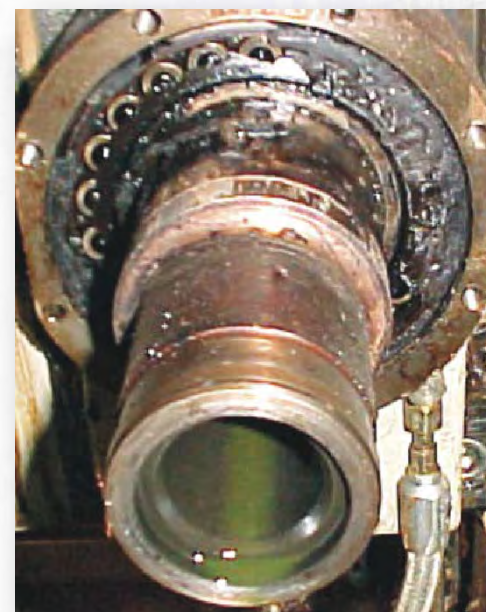
A visible oil drip preceded this bearing lock-up.
