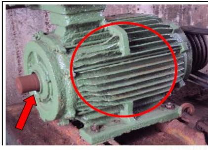
Calculated Maximum allowable surface winding area 70°C. Motor operating at least 35°C above allowable. Motor life diminished from 20 years to less than 2 years.
